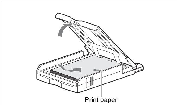
Riffle through the print paper before loading it with the printing surface (the side without imprinting) facing up. Make sure that the arrow on the protective sheet is pointing in the same direction as the arrow on the tray. You can load up to 25 sheets when using the UPC-X46 series and 30 sheets when using the UPC-X34 series.
